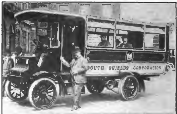
The Anderson Electric Car Co., Detroit, Mich., maker of Detroit electrics, has received orders from London for a number of buses similar to those already in use in that city. These buses, of the type illustrated above, are fitted with 60 A-8 Edison batteries capable of carrying the vehicle 50 miles on a charge. The capacity of each bus is thirty people
